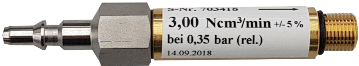
Figure 84: Test leak with Stäubli plug-in nipple
