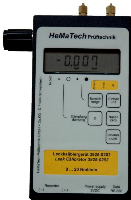
Figure 86: Leak calibration device
